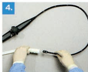
4. Slip the transducer via the applicator into the latexfree cover.
