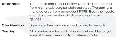
Standard needle is 17 gauge x 31 cm with 60 cm tubing – Order code SC1SE. Also available in other gauges or lengths, please state when ordering.
